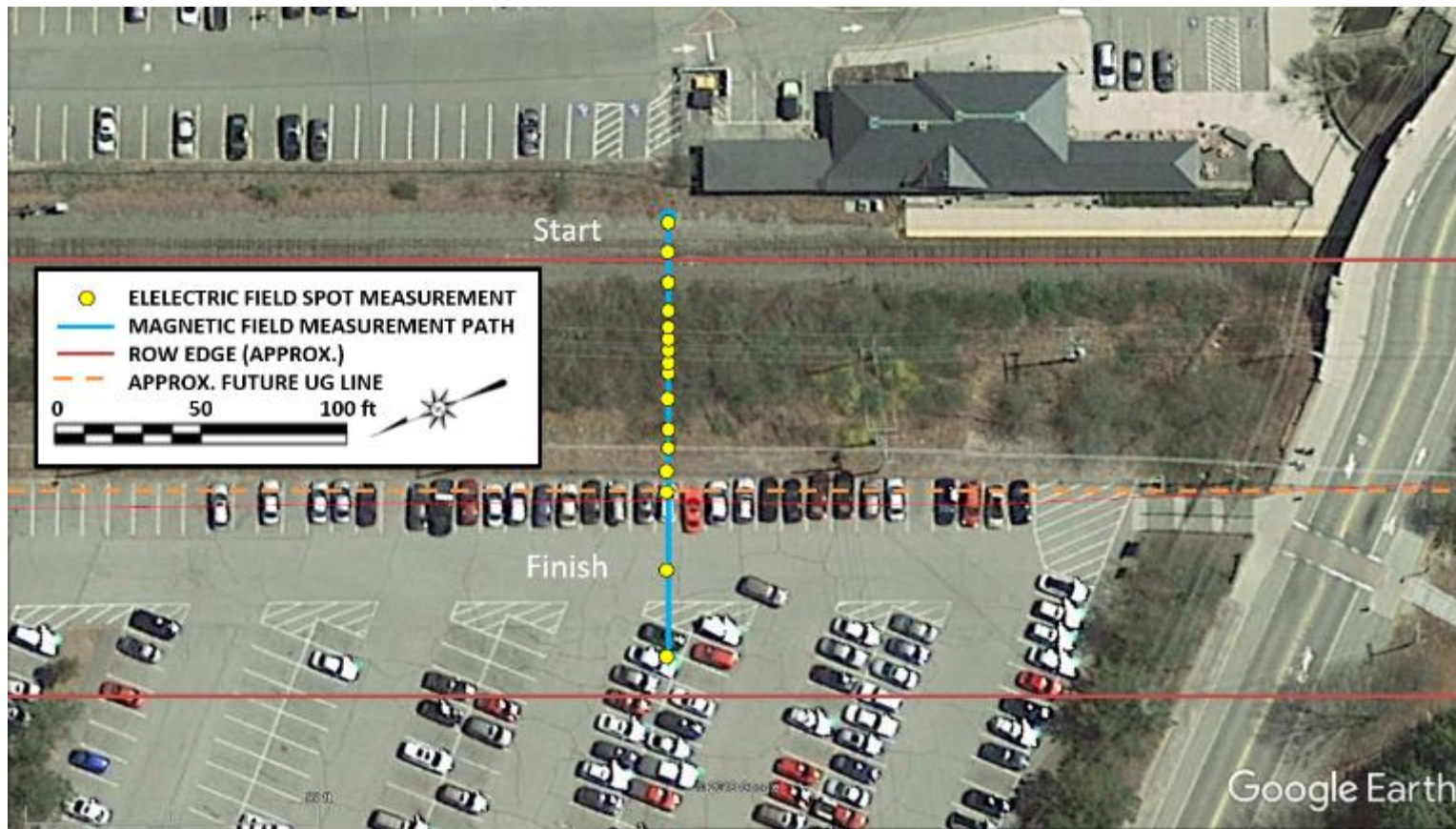
Figure C-2. Aerial photograph of measurement Site 2 (UNH Parking Lot A) showing the approximate location of the magnetic-field measurement path and electric-field spot measurements performed on July 21, 2020.
